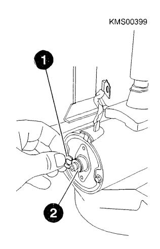
Disassembling commutator end shield
